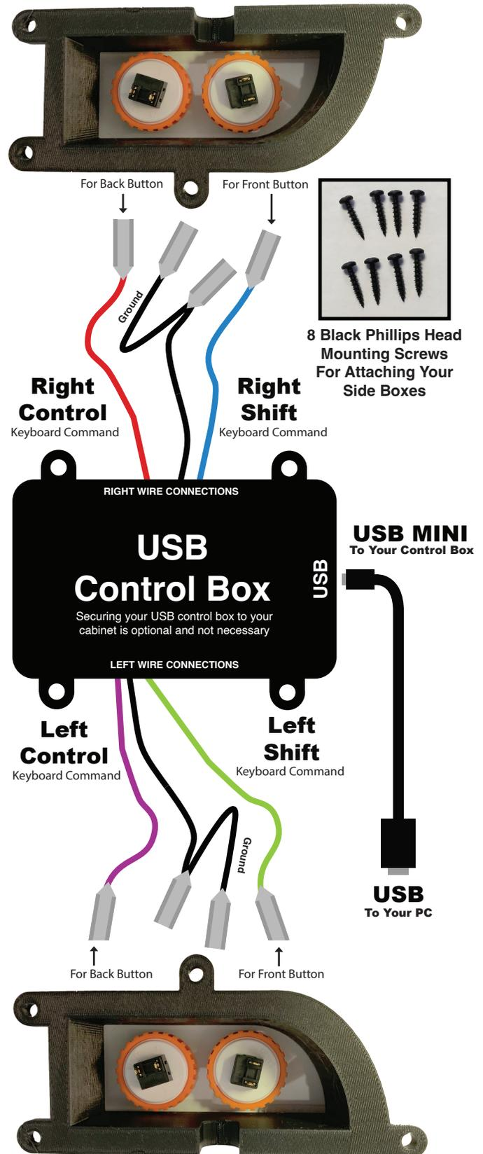
NOTE: IT DOES NOT MATTER WHICH PRONG THE COLORED WIRES ARE CONNECTED TO, AS LONG AS THEY ARE PLUGGED INTO THE CORRECT FRONT OR BACK BUTTON.
